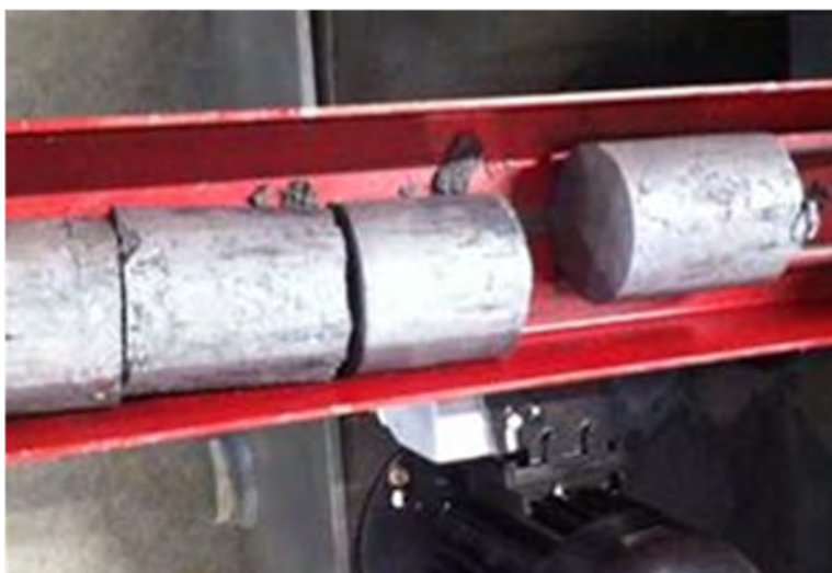
Figure 13-6 6 CLC Pilot Plant Lead Cement compacted as Briquettes
